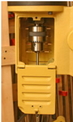
A pair of chuck access doors and the provided extended chuck key makes auger bit changes fast and easy. A chuck extender is included for using short-shanked chisels.
