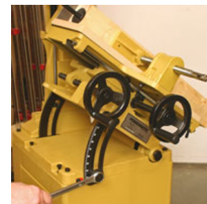
The entire table tilts up to 35-degrees in addition to the X/Y movements to make even complicated mortises easy to produce.
