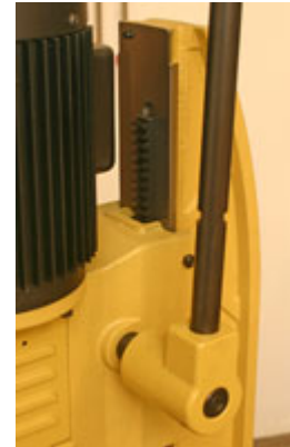
The rack and pinion drive combined with the 24"-long steel operating arm and repositionable hub make it easy to use the most comfortable stroke for the job at hand.
