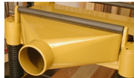
A dust shroud with a 5"-diameter discharge port handles moving the debris away from the cutterhead.
