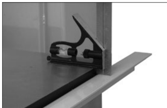
Figure 5: aligning rear rail
