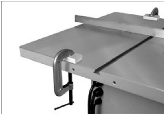
Figure 6-5: leveling extension wings, method 2
