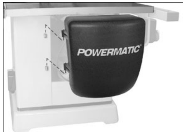
Figure 6-7: installing motor cover
